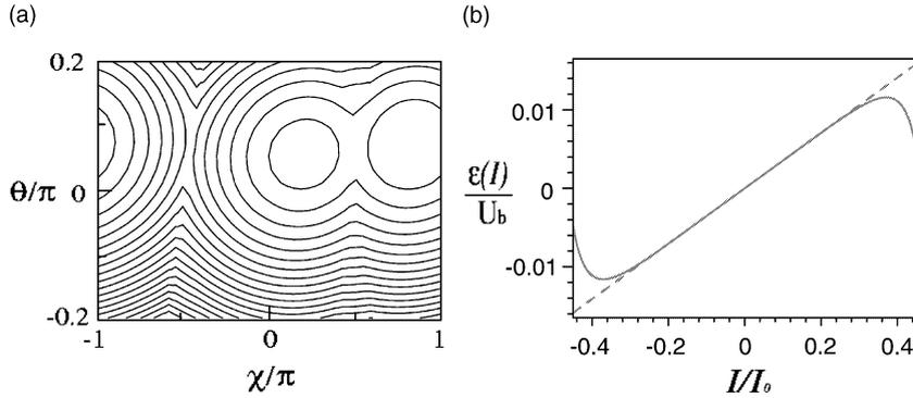
Fig. 3. (a) Contour plot of the free energy for the system of Fig. 2b at  $\mathcal{S} = 0.05$ . (b) Solid line is the energy bias as a function of the transport current, normalized to the barrier height, for the system of Fig. 2b. Dashed line is the linear approximation.
