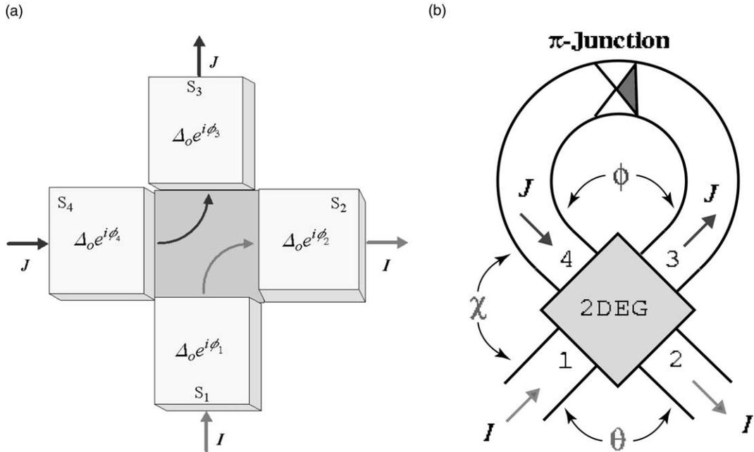
Fig. 1. Mesoscopic (a) four-terminal junction and (b) four-terminal SQUID. The  $\pi$ -junction is included in the ring to attain bistability.
