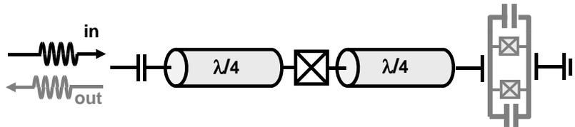
**Fig. 1.4** Coupled qubit-nonlinear resonator system. The transmon qubit is capacitively coupled to one end of the nonlinear resonator, while the other end is coupled to a  $50\Omega$  measurement line through which microwave pulses of amplitude  $\epsilon_p$  (resp.  $\epsilon_s$ ) and frequency  $\omega_p$  (resp.  $\omega_s$ ) drive the resonator (resp. the qubit).
