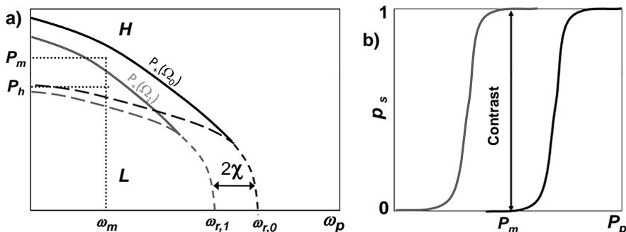
**Fig. 1.8** Principle of JBA readout. (a) Sketch of the stability diagrams of the NL resonator dispersively coupled to a transmon prepared in state  $|0\rangle$  (black) or  $|1\rangle$  (grey). (b) Sketch of the probability  $p_s$  to measure the resonator in state  $H$  for qubit initially in  $|0\rangle$  (black) or  $|1\rangle$  (grey).
