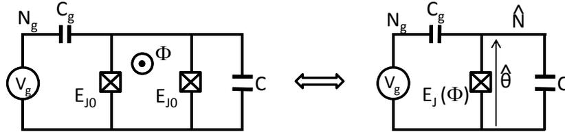
**Fig. 1.3** Circuit model of a split Cooper-pair box made of a superconducting loop including two Josephson junctions of Josephson energy  $E_{J0}$  threaded by a flux  $\Phi$ , shunted by a capacitor  $C$ , and charge-biased by a voltage source  $V_g$  through a gate capacitor  $C_g$  yielding a charge bias  $N_g = C_g V_g / (2e)$ .
