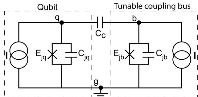
FIG. 1. A pair of capacitively coupled CBJJ qubits.
