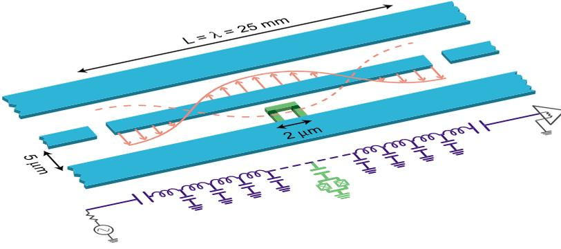
FIG. 1. (Color online) Schematic layout and lumped element version of the circuit QED implementation. A superconducting charge qubit (green) is fabricated inside a superconducting one-dimensional transmission line resonator (blue).
