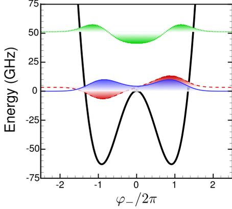
FIG. 4. (Color online) Cut along the  $\varphi_+=0$  axis of the double well potential of the flux qubit with the first (full blue), second (dashed red), and third (dotted green) eigenstates for qubit parameters  $E_{J1}=259$  GHz,  $\alpha=0.8$ , and  $E_J/E_C=35$  with  $\Phi_{\text{ext}}=\Phi_0/2$ .
