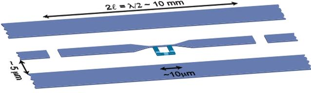
FIG. 1. (Color online) Schematics of a three-junction flux qubit directly connected to the center conductor of an inhomogeneous superconducting transmission-line resonator.
