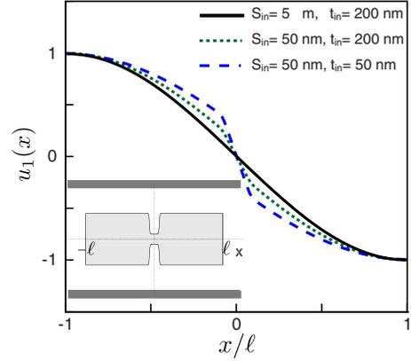
FIG. 2. (Color online) First mode (normalized to 1) for aluminum transmission-line resonators with the different constriction parameters listed in Table I. As the central line is reduced in cross section, the slope of the flux field increases inside the constriction. The inset shows the geometry of the constriction in the center conductor of the resonator.
