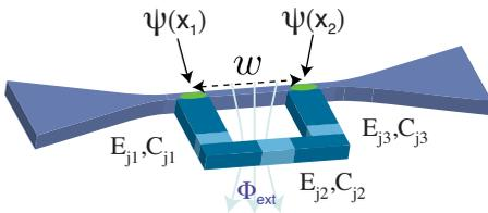
FIG. 3. (Color online) Closeup of the flux qubit fabricated at the location of the constriction. The qubit is attached at positions  $x_1$  and  $x_2$  on the resonator.  $\Phi_{\text{ext}}$  is an externally applied flux. A large Josephson junction inserted in the center conductor of the resonator between  $x_1$  and  $x_2$  can lead to stronger coupling.
