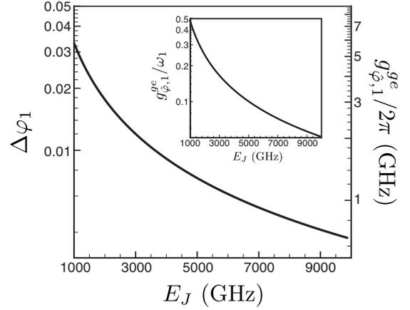
FIG. 5. Flux bias  $\Delta\varphi_1$  and resultant qubit-resonator coupling energy  $g_{\varphi_1}^{ge}$  as calculated from Eq. (3.12) induced by a Josephson junction placed in the center of a homogenous aluminum transmission-line resonator (see Table I) as a function of the Josephson energy  $E_J$ . The inset shows that the qubit-resonator coupling energy can reach several tens of percent of the resonator frequency. Qubit parameters are given in the text.
