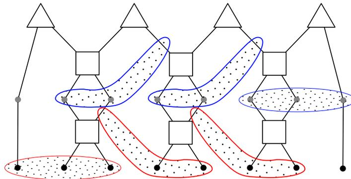
**Figure 3.** Identification of the disentangles using two successive sweeps of the chain. Dotted regions cover particles on which brute-force tomography is performed. The first sweep (red dotted regions) finds unitaries starting from the left end of the chain. Those unitaries will be used as initial guesses for the second sweep (blue striped regions) that starts from the right end of the chain.
