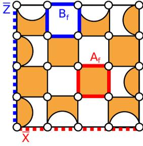
FIG. 1. Layout of the surface code where qubits are located at vertices. Orange faces represent  $A_f$  checks and white faces represent  $B_f$  checks. The logical  $\bar{Z}$  operator is a product of  $Z$  along the dashed blue and the logical  $\bar{X}$  operator is a product of  $X$  along the dashed red line.
