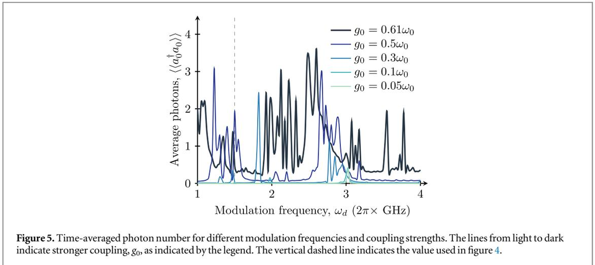
**Figure 5.** Time-averaged photon number for different modulation frequencies and coupling strengths. The lines from light to dark indicate stronger coupling,  $g_0$ , as indicated by the legend. The vertical dashed line indicates the value used in figure 4.
