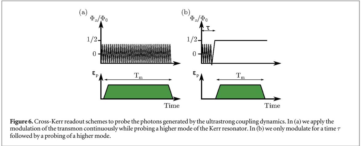
**Figure 6.** Cross-Kerr readout schemes to probe the photons generated by the ultrastrong coupling dynamics. In (a) we apply the modulation of the transmon continuously while probing a higher mode of the Kerr resonator. In (b) we only modulate for a time  $\tau$  followed by a probing of a higher mode.
